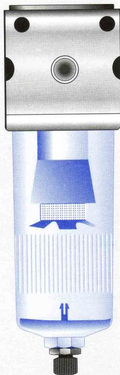
Standard filters of compact block design in two sizes with connecting threads from G1/4 to 3/4 . Facilities on both sides for flange mounting of further units. Direct mounting or bracket mounting on housing. Plastic bowls (polycarbonate) with optional metal protective casings or metal bowls with sight glass for higher pressures and temperatures.
